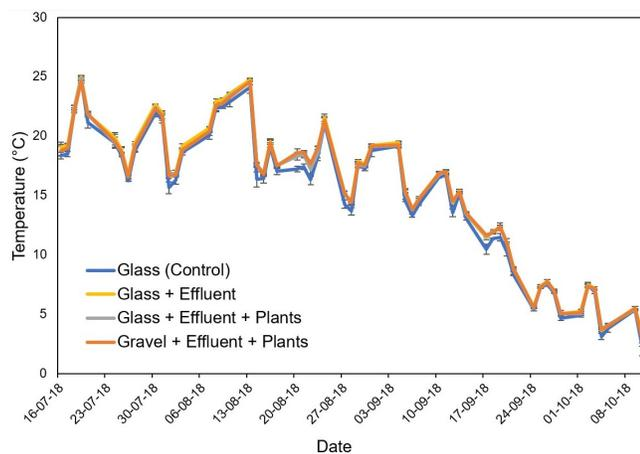
Figure S1. Mean temperature ( $^{\circ}\text{C}$ ) of treated mesocosms at the Prairie Wetland Research Facility (PWRF). Temperature values were averaged across replicates ( $n=3$ ) for each of the four treatments (control, gravel, plant glass, and glass). Measurements were made using a YSI 6600 V2 Sonde every weekday morning from July 16<sup>th</sup>, 2018 to October 10<sup>th</sup>, 2018. Error bars represent standard deviation.
