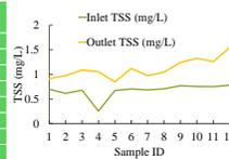
Fig 5. TSS and turbidity are significantly higher in the outlet than in the inlet.
