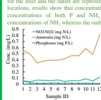
Fig 6. Conc. of P, NO<sub>3</sub>/NO<sub>2</sub> and NH<sub>4</sub> for the inlet filtered sub-samples
